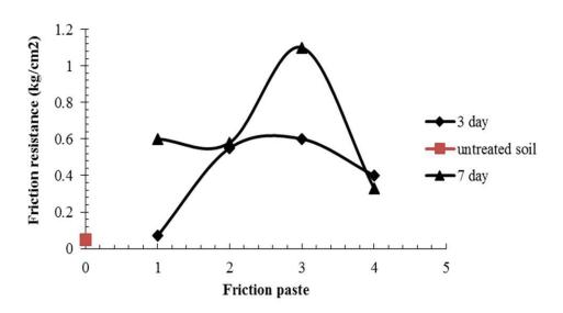
Figure 6: Value of soil-pile friction resistance for each mixture for 3 and 7 days curing period
